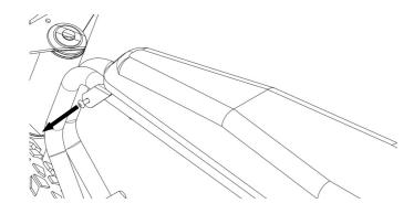
STEP 3: Place left sidepanel and hold it in its mounting position.
