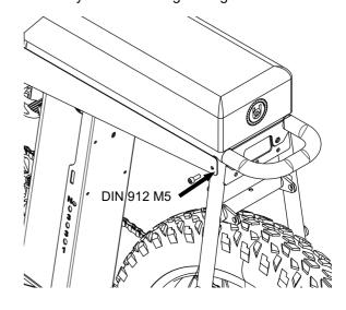
STEP 5: Screw back the seat hinge screw from STEP1 ensuring hole in the panel, seat hinge and frame threaded hole are all aligned. Do not tighten the screw completely.
